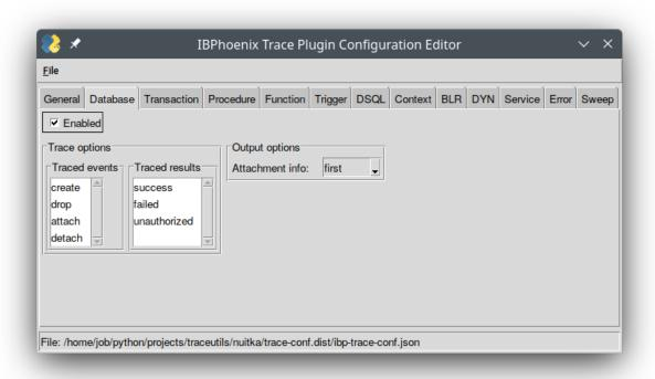
Fig. 3: The second tab is for setting of *database events*.
