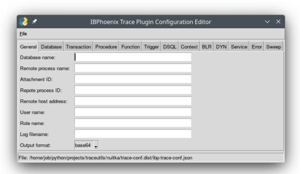
Fig. 1: The first tab is for setting of general filters.
