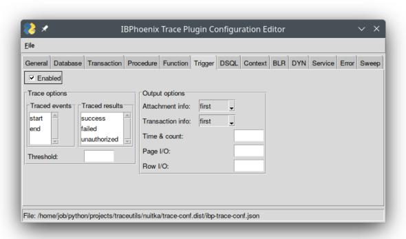
Fig. 7: The sixth tab is for setting of *trigger events*.
